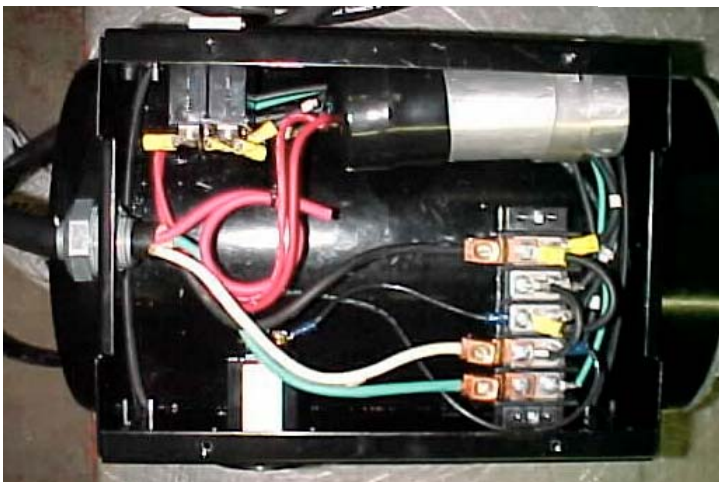
120 VAC connections 1&3 joined 2&4 joined
